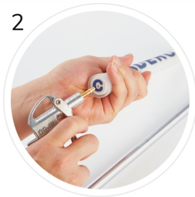
Please attach our recommended air gun to the grip end.
