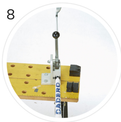
Please make sure that the grip is installed straight.
